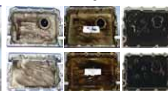
Kixx HD1 15W-40 81,000 Km Oil Drains A : 81,000 Km Oil Drains B : 48,000 Km Oil Drains
